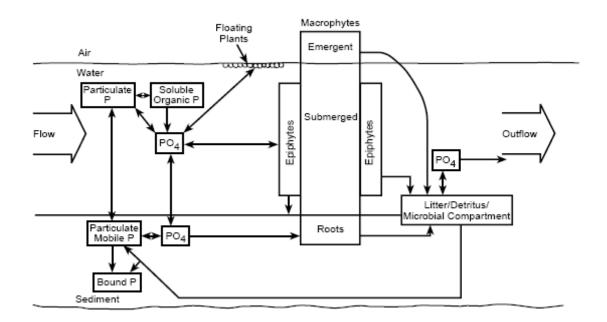
Figure 5 – Phosphorus transformations in a FWS wetland (EPA, 1999).
