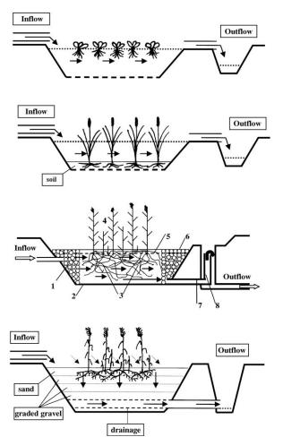
Figure 1 – The various types of constructed wetlands (Vymazal, 2006).
