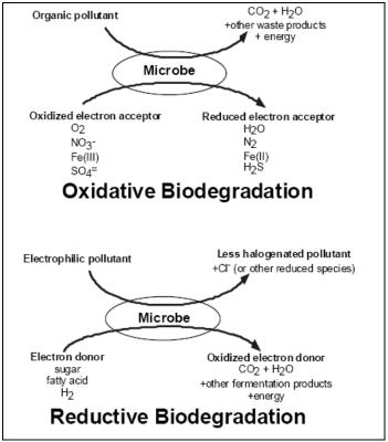
Figure 1: General Process of Organic Contaminant Degradation (Rockne and Reddy, 2003)
