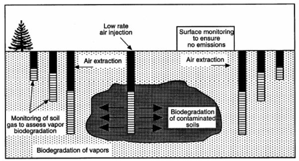
Figure 5: Typical Bioventing Operation (Rockne and Reddy, 2003)
