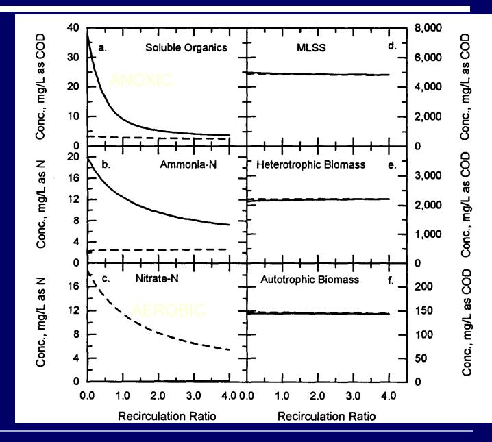
Solid lines indicate the anoxic (first) reactor and the dashed indicate The second (aerobic) reactor.
