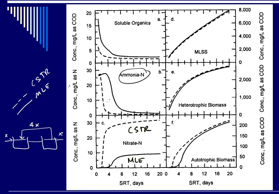
Dashed lines indicate performance of a single CSTR of the same volume as the anoxic and aerobic reactors.
