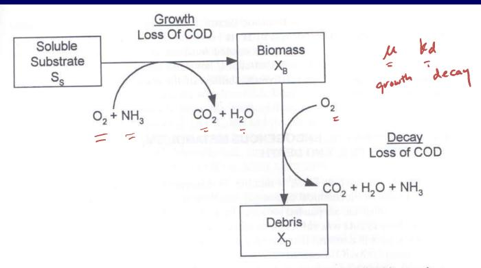
**Figure 3.5** Schematic representation of the traditional approach to modeling biomass decay and loss of viability.
