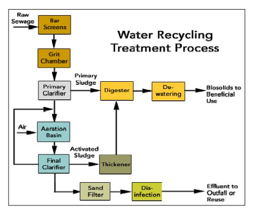
Figure 7: San Antonio Water Recycling Treatment Process (SAWS, 2006)
