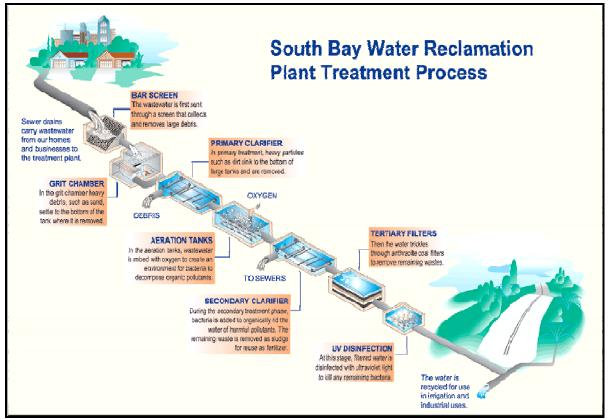
Figure 6: South Bay Water Reclamation Plant Treatment Process (The City of San Diego, 2006)
