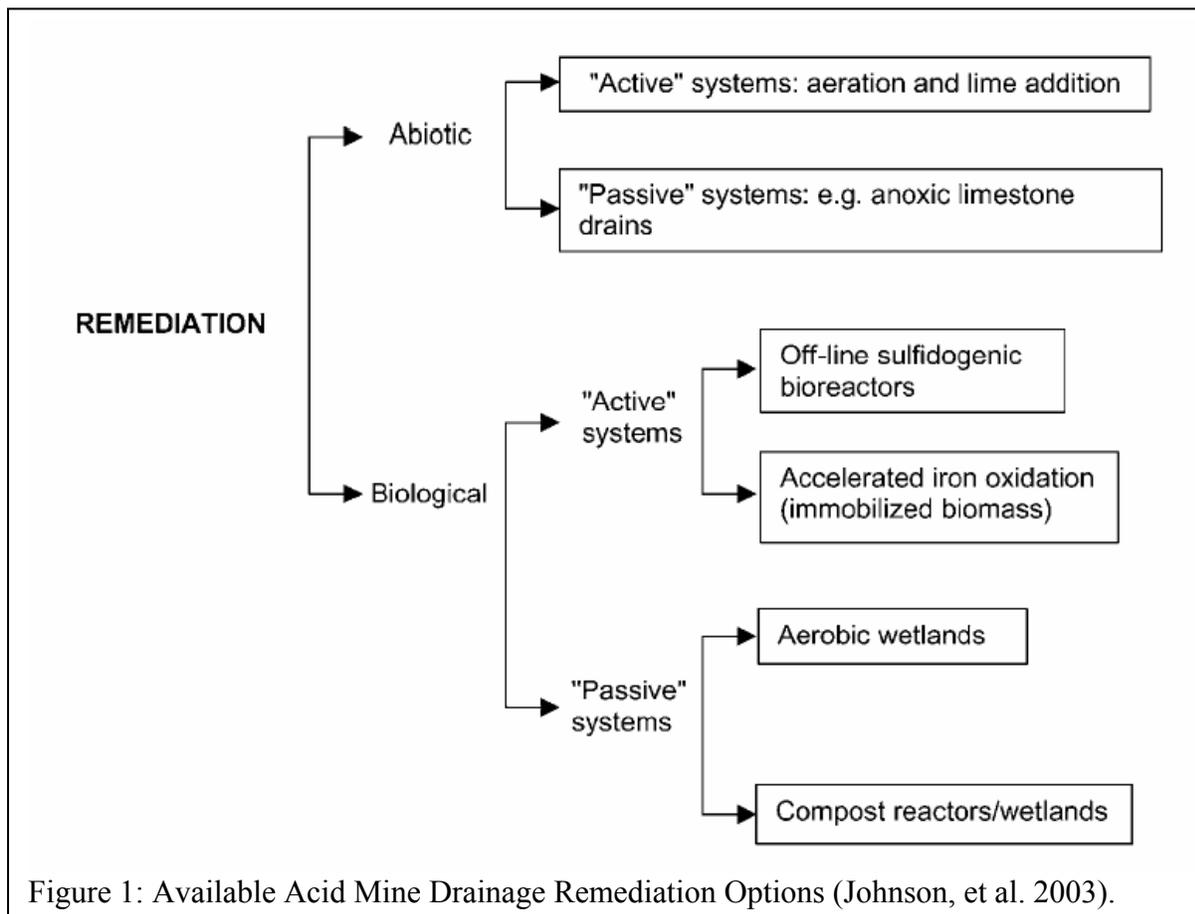
Figure 1: Available Acid Mine Drainage Remediation Options (Johnson, et al. 2003).
