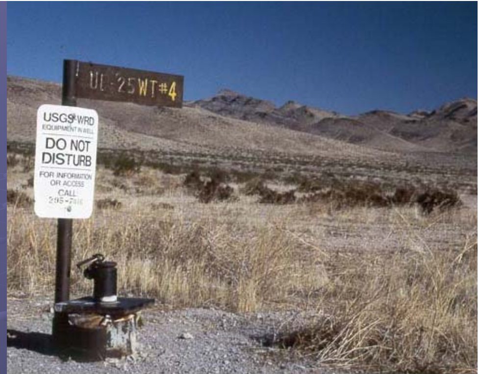
Monitoring Well UE-25 WT#4, Water level about 438 meters (1437 feet) deep Photo by USGS
