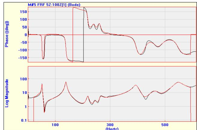
Figure 4 Typical FRF and Fit Function Overlaid.
