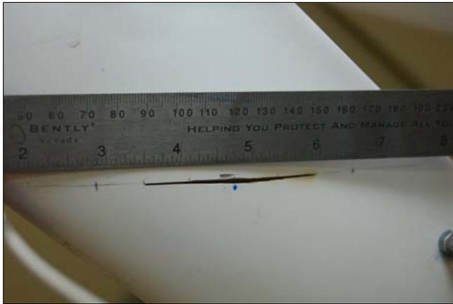
Figure 6 Surface Crack
