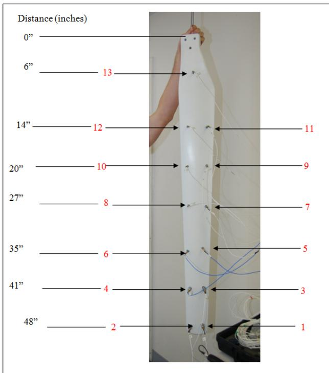
Figure 2 Accelerometer Locations.
