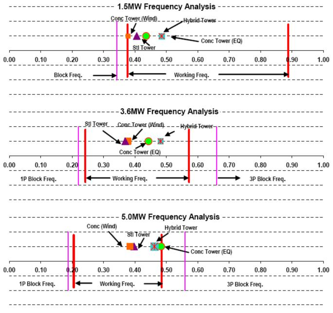
Figure 4.4. Operational frequency ranges for 1.5-, 3.6-, and 5.0-MW turbines
