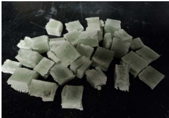
Figure 2. Cubes of Fiberglass Coarse Aggregate.
