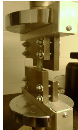
Figure 6. Device designed to clamp and hold samples to Instron plates during compression.
