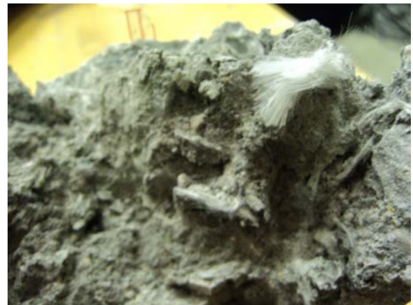
Figure 10. Clump of glass fiber along fracture.
