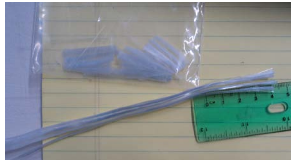
Figure 4. Virgin glass fibers cut from unidirectional strands.
