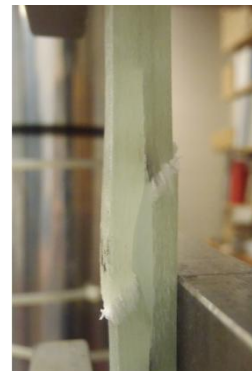
Figure 16. AR 12 sample clamped into place during fatigue testing. The illustration shows a failure around the wave.
