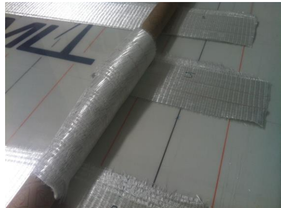
Figure 34: Dramatic example of helical winding. The fabric does not stay at the same place on the roll for straight fabric.
