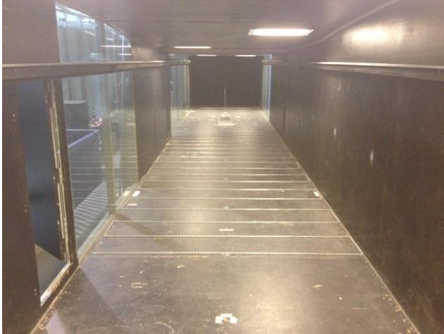
Figure 1. Test section of the wind tunnel with chains as roughness elements
