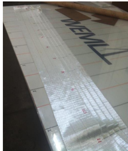
Figure 24: Two adhesive test showing both waves at the ends of the fabric within the adhesive
