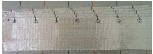
Figure 23: Effect of rolling in the "number 1" direction. Straight lines before, staggered afterwards.
