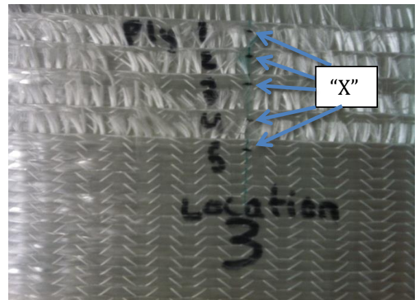
Figure 13: “X” spots where the measurements would be recorded. Notice the small black lines on the vertical green line.
