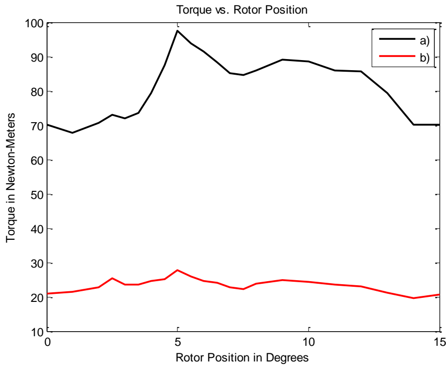
Figure A3. Comparison torque profiles with a) modified winding areas and b) reduced current density in the modified winding areas
