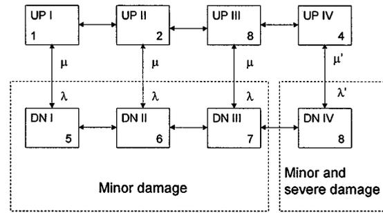
Fig. 18. Reliability model for wind turbine.
