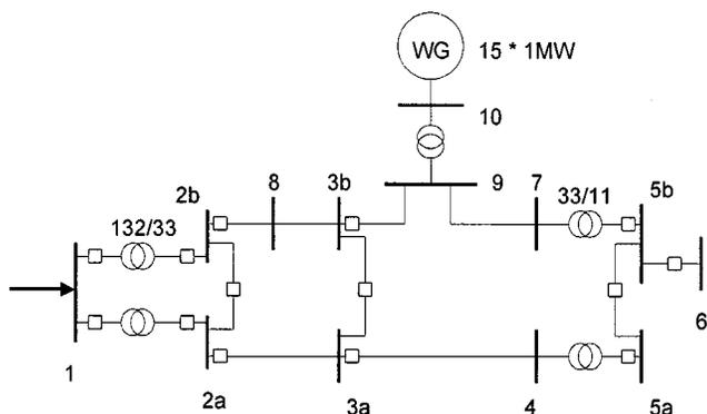
**Fig. 20.** Meshed system with wind farm.
