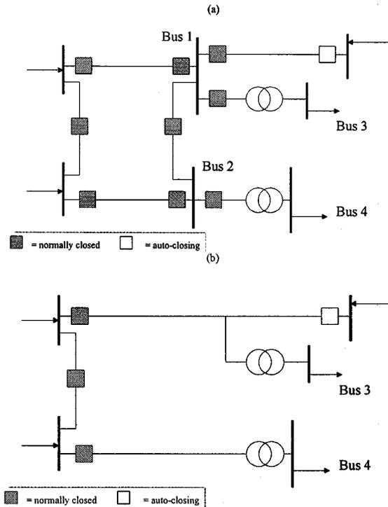
**Fig. 21.** Network to consider asset replacement, (a) before changes and (b) after changes.
