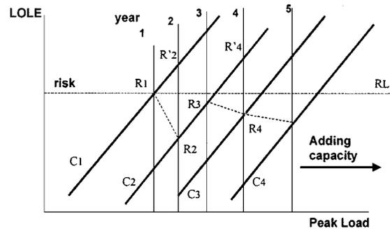
Fig. 7. Possible generation expansion plan.
