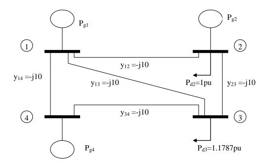
Fig. 1: One line diagram for example system
