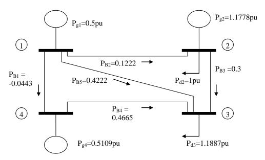
Fig. 7: Flows for case 2 with 1 MW increase in P<sub>d3</sub>
