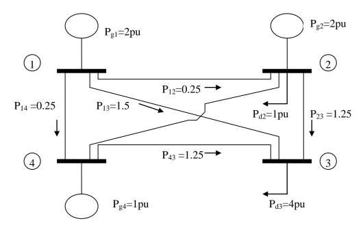
7. Using the same system you analyzed in problem 1, set up the optimal power flow as a linear program. Assume the objective function is exactly the same as used in the example in class, i.e.,
