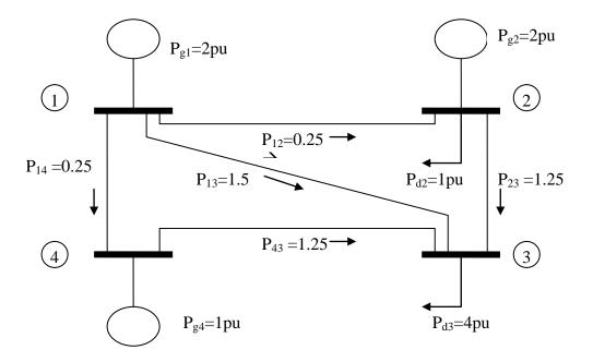
Fig. 3: Computed flows for four-bus network used in example
