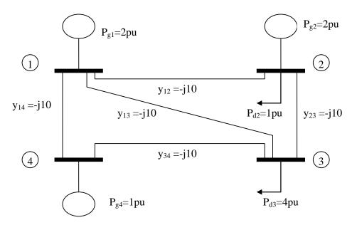
Fig. 2: Four-bus network used in example
