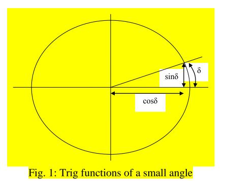
In Fig. 1, it is clear that as the angle  $\delta = \theta_k \cdot \theta_j$  gets smaller and smaller, the cosine function approaches 1.0.
