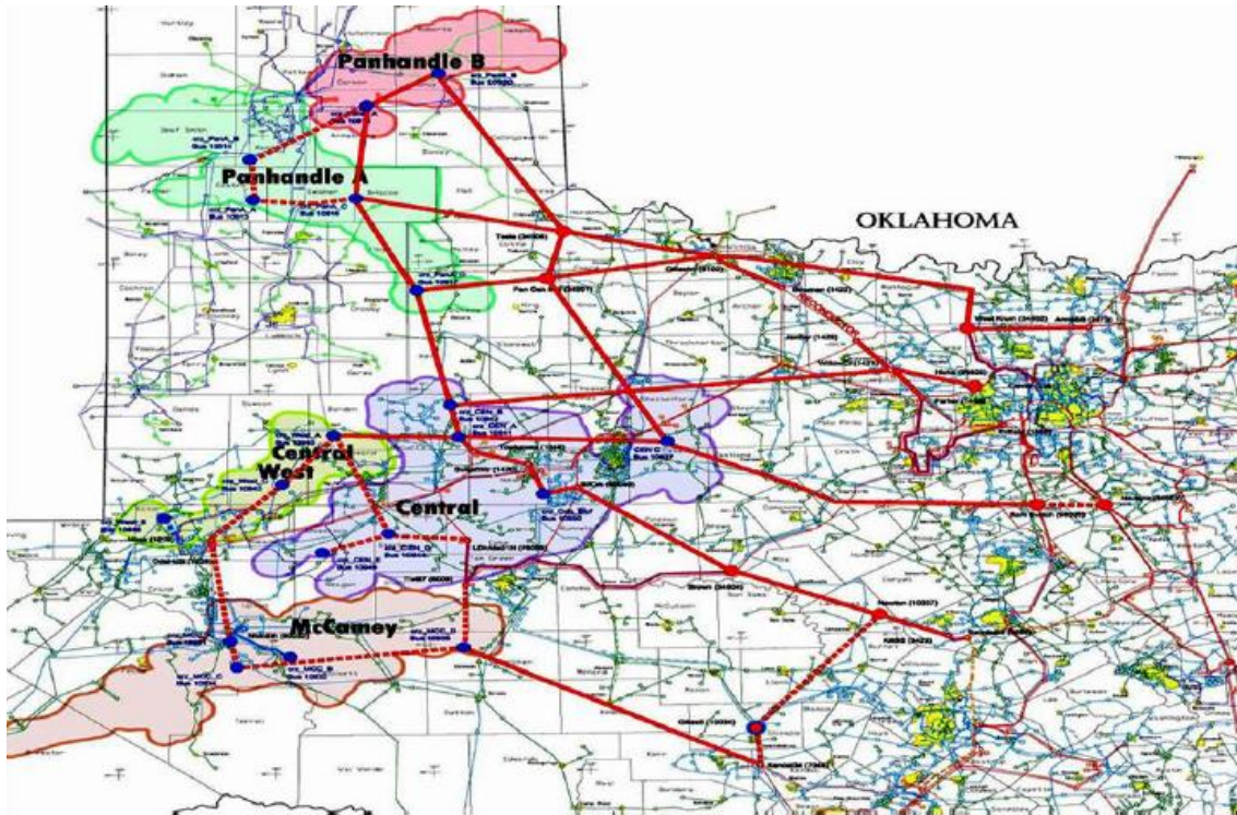
Figure 7-6: The 345 kV CREZ system
