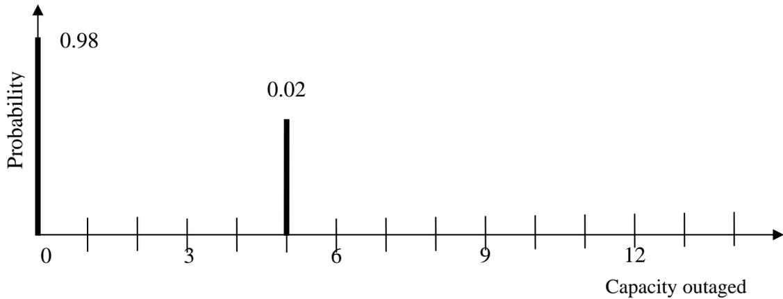
Fig. U19.9: pmf for 5 MW Capacity Outage
