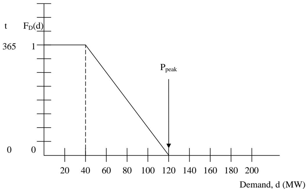
Fig U19.15a: Load shape curve for example [1]
