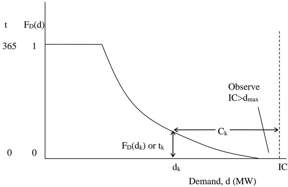
Fig. U19.13: Relationship between capacity outage, load model [1]
