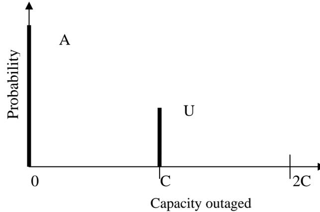
Fig. U19.3: pmf for Capacity Outage of One-Unit Example
