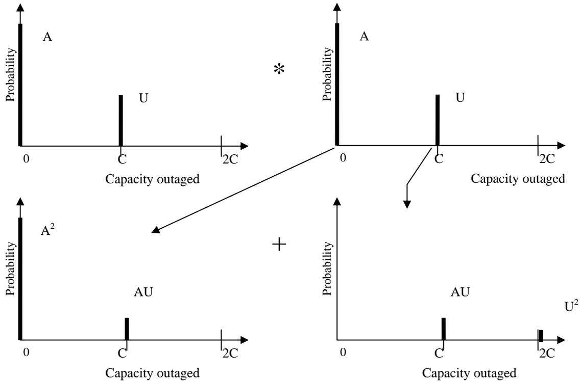
Fig. U19.4: Convolution of Generator Outage Capacity pmfs
