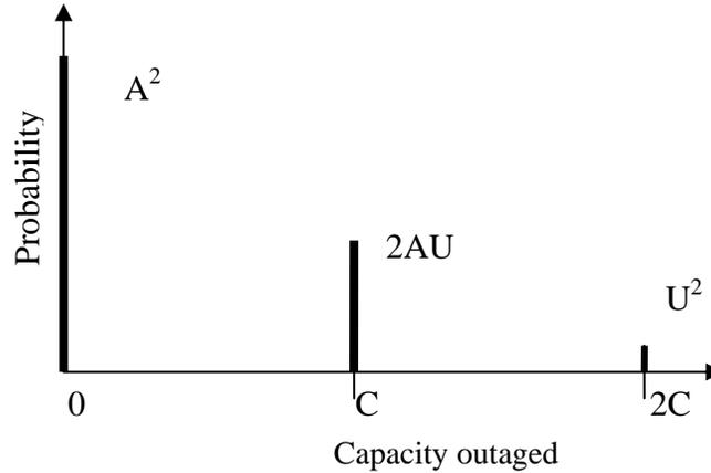
Fig. U19.5: pmf for Capacity Outage of 2 Unit Example
