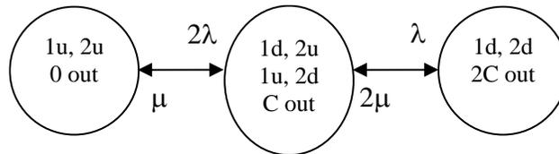
Fig. U19.7: Reduced State Space Model for 2 Unit System
