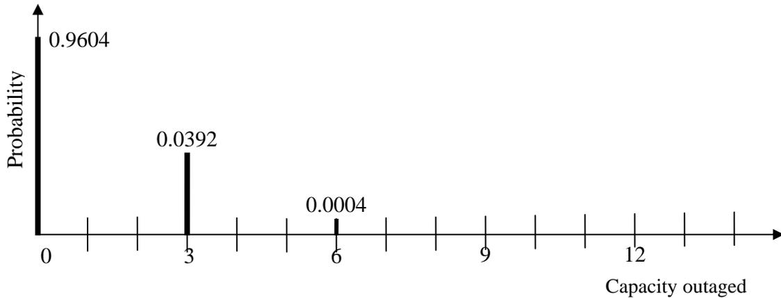
Fig. U19.8: pmf for Capacity Outage of Convolved 3 MW Units
