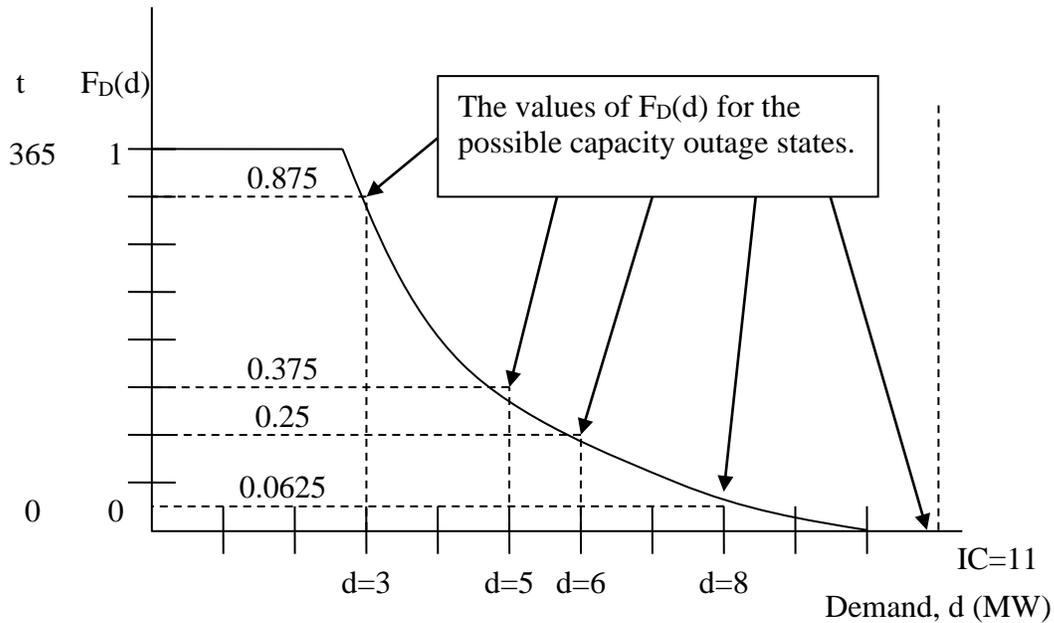
Fig. U19.14: Load shape curve for example
