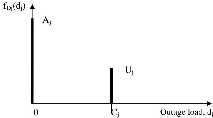
Fig. U19.20: Two state generator outage model
