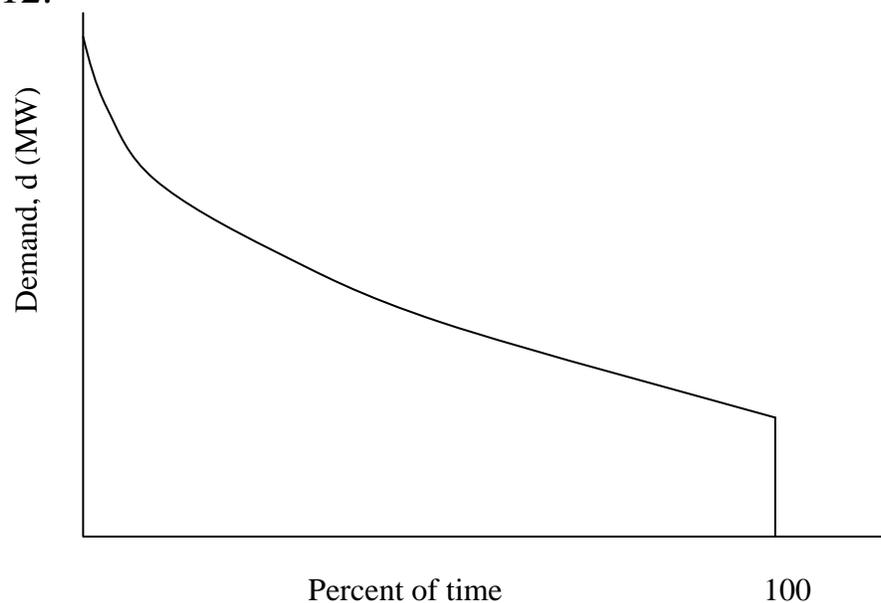
Fig. U19.12: Load duration curve
