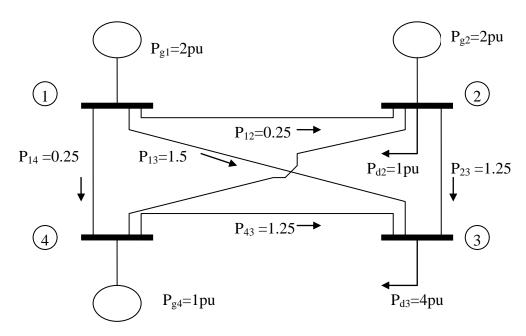
2. Using the same system you analyzed in problem 1, set up the optimal power flow as a linear program. Assume the objective function is exactly the same as used in the example in class, i.e.,
