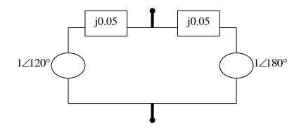
The Thevenin impedance is j.05/2=j.025. The Thevenin voltage is found from KVL:  $1 < 120^{\circ} - jI(0.1) = 1 < 180^{\circ} \rightarrow I = (1 < 120^{\circ} - 1 < 180^{\circ})/j0.1 = 10 < -30^{\circ}$ .
