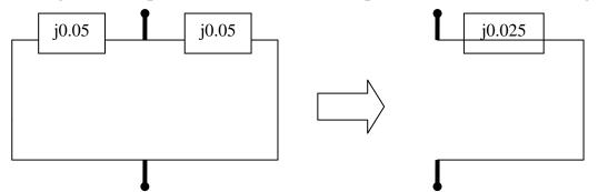
Since this is a line-to-line fault, we do not need the zero-sequence network, but need only to connect the positive and negative sequence networks as shown below.
