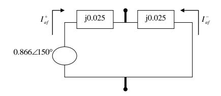
The fault positive sequence current is computed as
