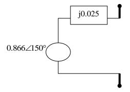
The negative sequence network appears as below, with the dark lines indicating the fault point, and the Thevenin equivalent is shown to the right.
