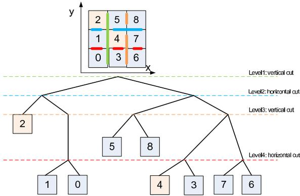
Fig. 4. An example of partition tree for  $3 \times 3$  expansion region, the vertical cut line is first applied. The bin 2 and 4 are occupied by fixed macros
