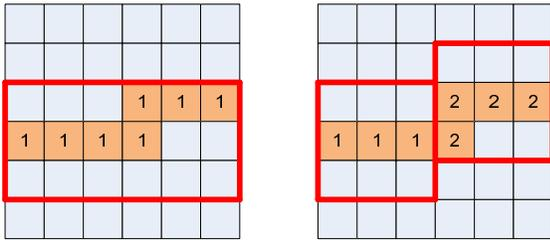
Fig. 2. Imposing upper bound on the number of bins in a hotspot. The overflow bins are coloured , the boundary of expansion region is marked by the red bold line.
