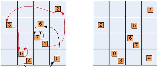
Fig. 5. An example of two move chains, the left figure shows the original cell position and move chains, the right figure shows the new cell position after movement.
