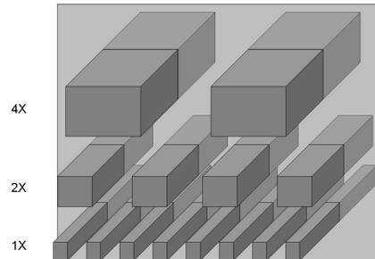
Fig. 3. Layer assignment for 65nm and beyond.
