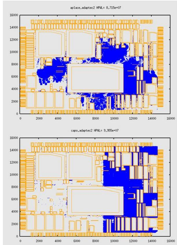
Fig. 1. Solution by APlace (top) and Capo (bottom) for adaptec2 in ISPD 2005 placement contest.
